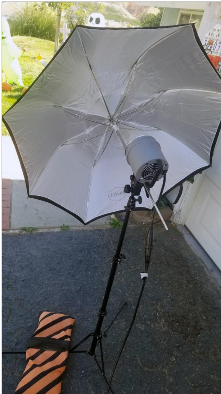
The setup to 'bounce' a strobe light off a specially designed umbrella (above).
